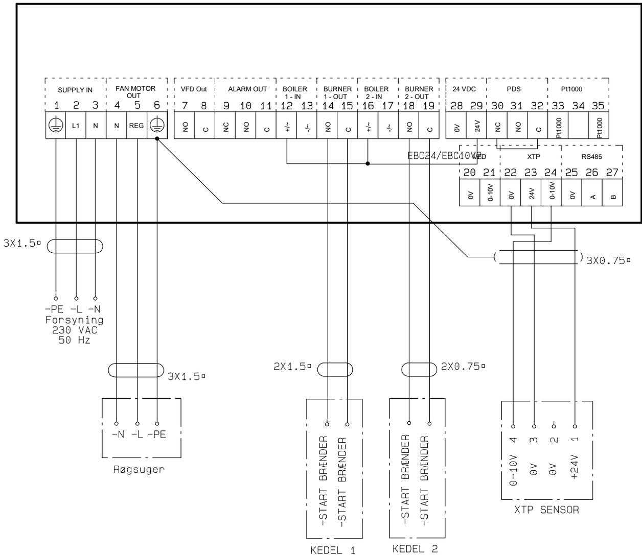
This example shows how to connect the EBC24 if you require continuous operation of the chimney fan:
