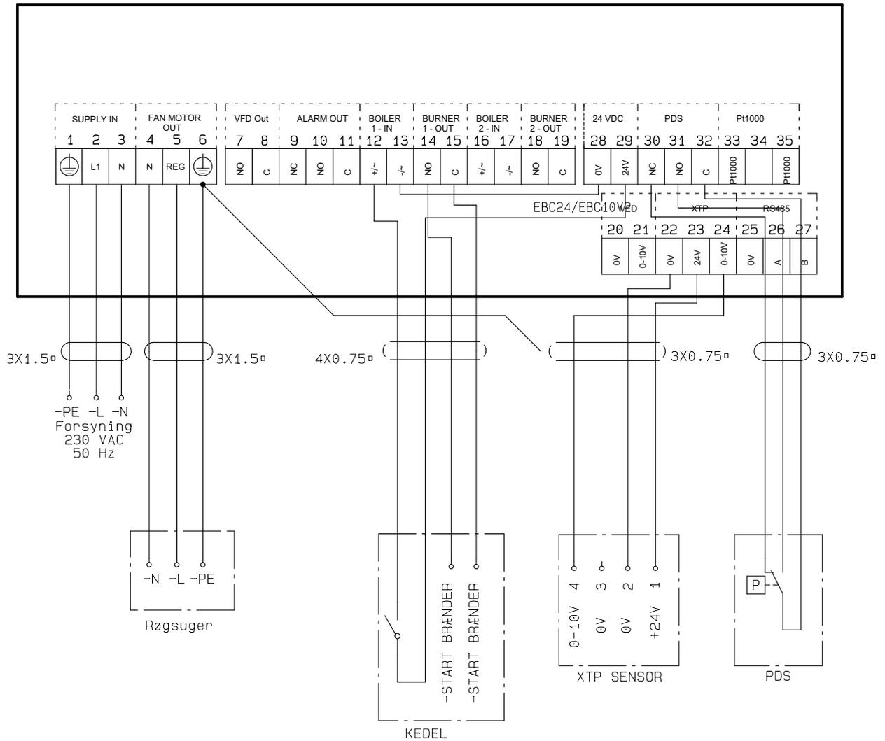
This example shows how to connect a PDS to EBC24. The PDS supplies extra monitoring
