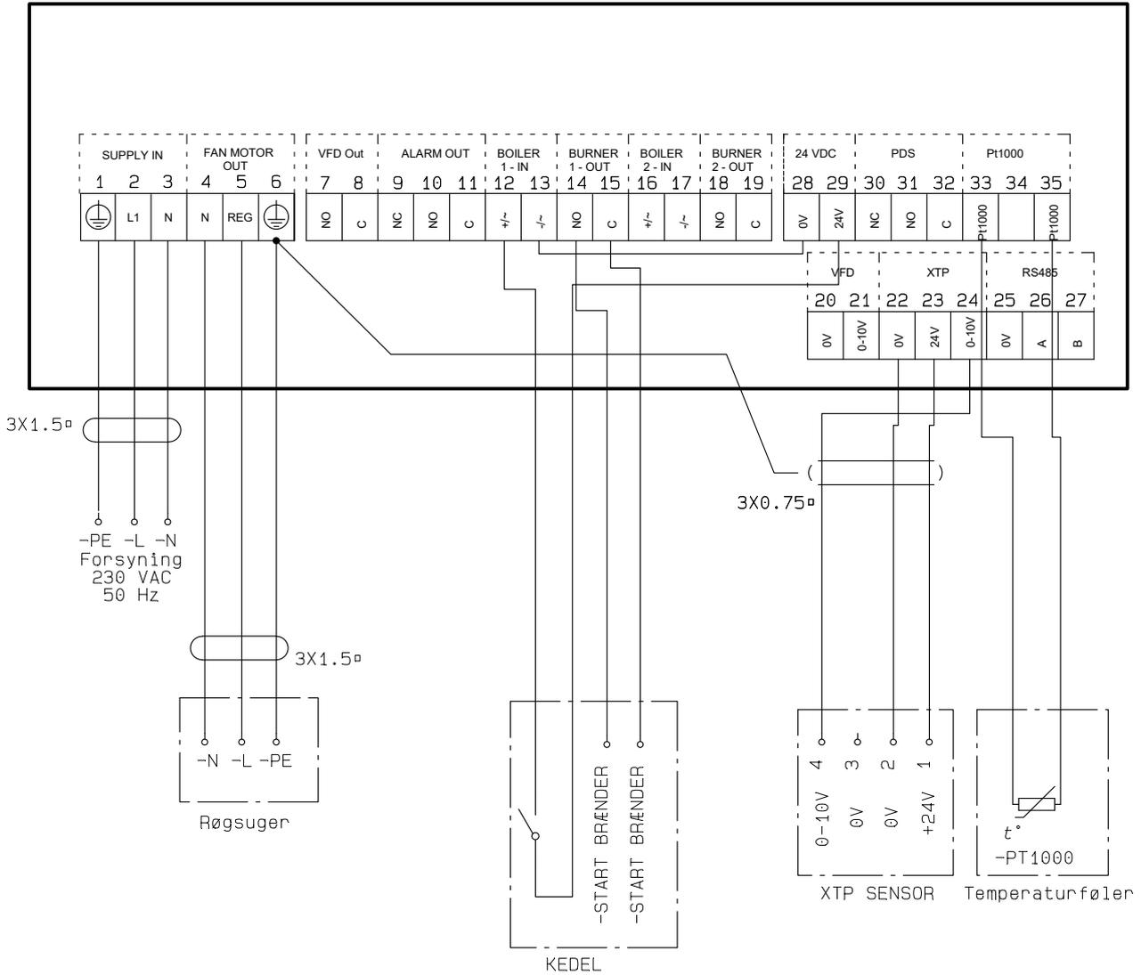
This example shows how to connect a potential free contact to the EBC24 to start/stop the fan:
