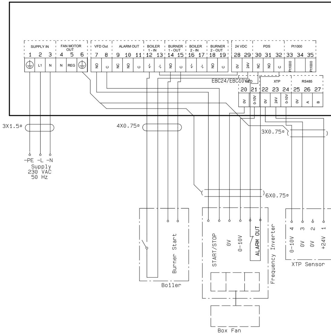
This example shows which inputs/outputs on the EBC24 need to be connected to the frequency converter/MPR-relay:
