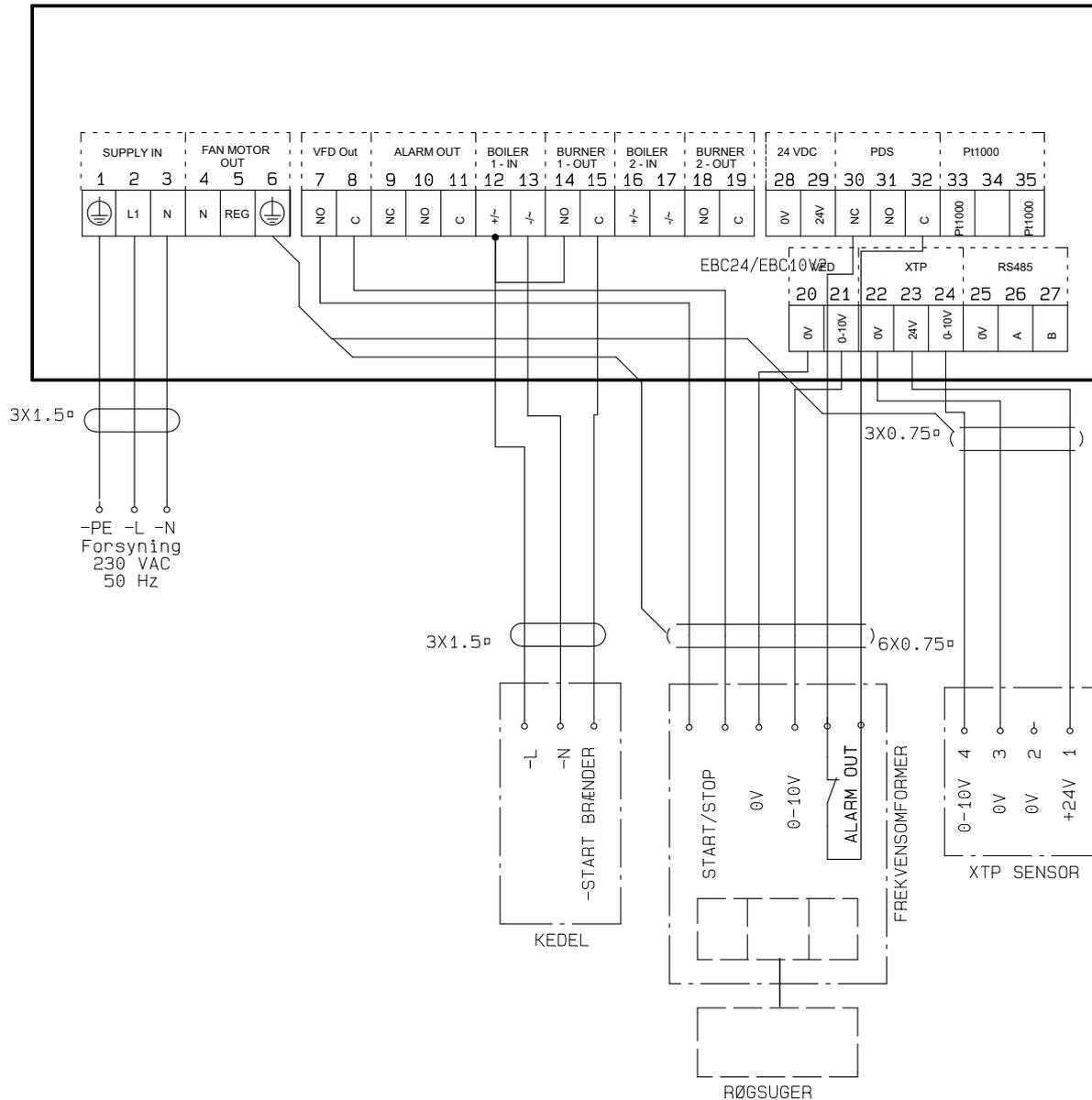
This example shows which inputs/outputs on the EBC24 need to be connected to the frequency converter, when one is used to control the chimney fan:
