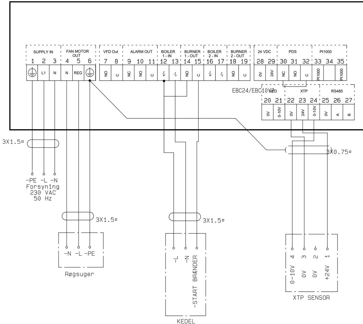
This example shows how to connect a voltage signal (18-230 V AC/DC) to EBC24 to start/stop the chimney fan.
